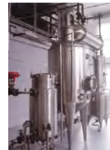
WZS单效外循环真空浓缩回收器(自动防爆型) WZ single effect external circulation vacuum cream reclaim concentrator
